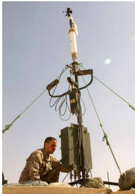
Military WEATHERPAK® with additional visibility sensor
