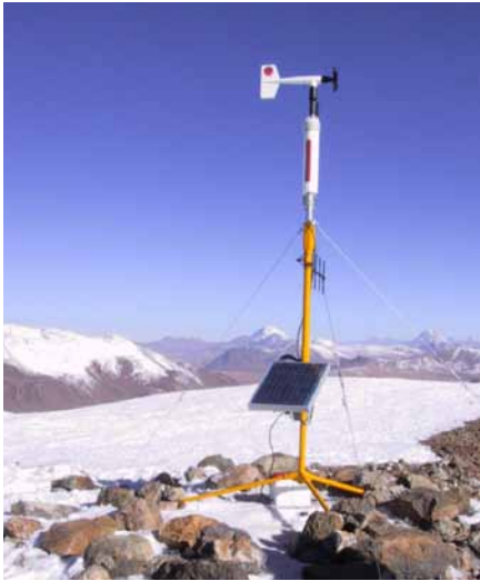
Solar powered WEATHERPAK® in Atacama, Chile
